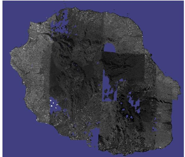
Figure 4: 3D reconstruction of the whole Réunion island obtained with s2p from 9 Pléiades stereo datasets. The points are colored with the original panchromatic channel of the respective reference images. The input images were downsampled 16 times.
