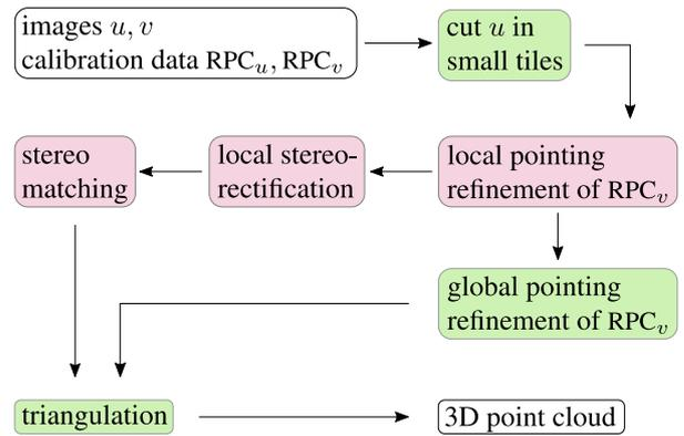
Figure 1: Stereo pipeline overview. The input is a pair of images with their respective rational polynomial camera models, and the output is a digital elevation model given as a georeferenced 3D point cloud. Green blocks are applied to the whole images, while pink blocks are applied on small independent tiles. They can be processed in parallel.
