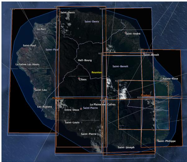
Figure 3: Coverage of the Réunion island by Pléiades stereo images. Eight stereo pairs and one tri-stereo dataset were used. Each rectangle corresponds to a dataset. The larger image has dimensions of approximately  $40\,000 \times 120\,000$  pixels.
