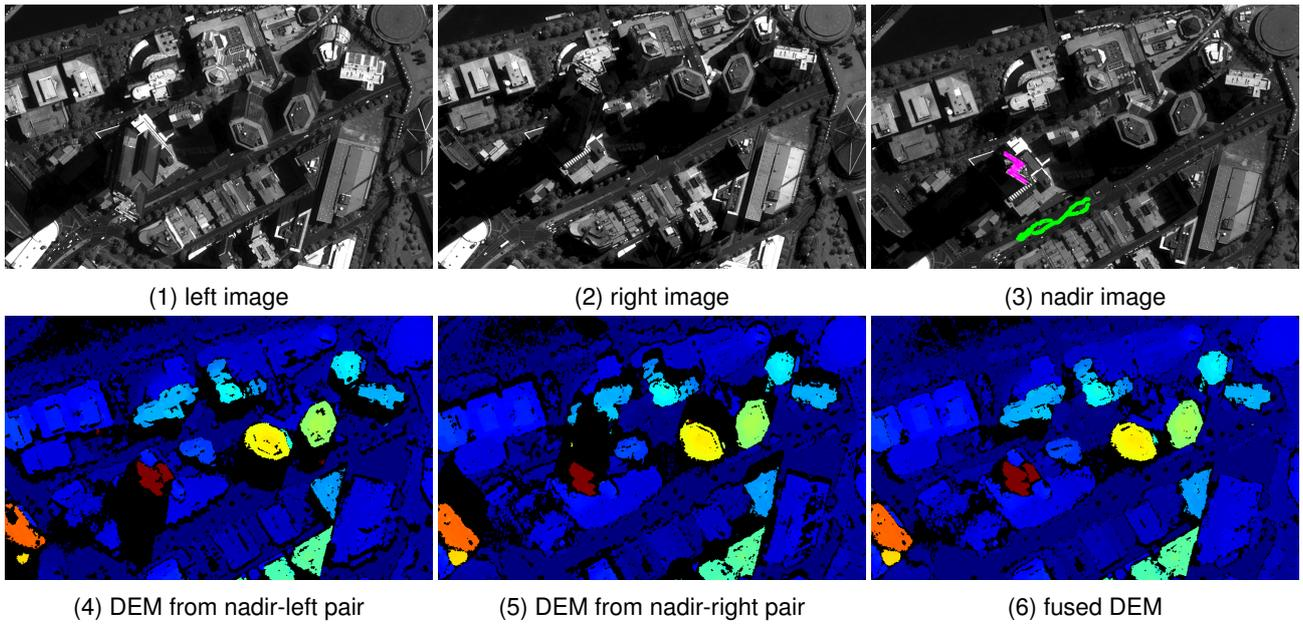
Figure 2: Tri-stereo Pléiades images of Melbourne (1-3), the roof and street areas used for the evaluation are shown in (3). The elevation maps obtained by taking only two images are shown in (4) and (5), while (6) corresponds to the fusion with outlier filtering. Black areas represent rejected pixels.
