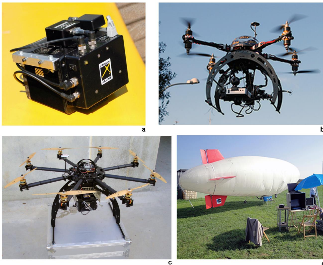
Figure 4: Oben's material and fleet examples ( www.oben.it ), a. first prototype of YellowScan LiDAR ( www.lavionjaune.fr ); b. Multi-rotor drone OB-I; c. Multi-rotor drone OB-II with YellowScan LiDAR onboard; d. 10 m length dirigible (Photos by Oben srl).
