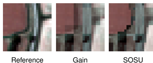
Figure 19 – Extract from A3 better reconstructed with SOSU than with Gain (4 m spatial resolutions).
