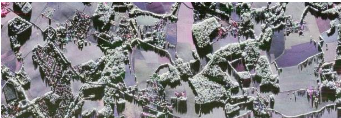
Figure 10 : X-Band Polarimetric image at grazing incidence angle (80°) acquired during the MENAS-BIS campaign.
