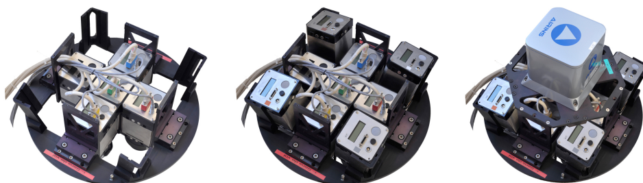
Figure 2 : From the left to the right: CAMv2 system in medium format, in large format and in its large format equipped with an IMU.
