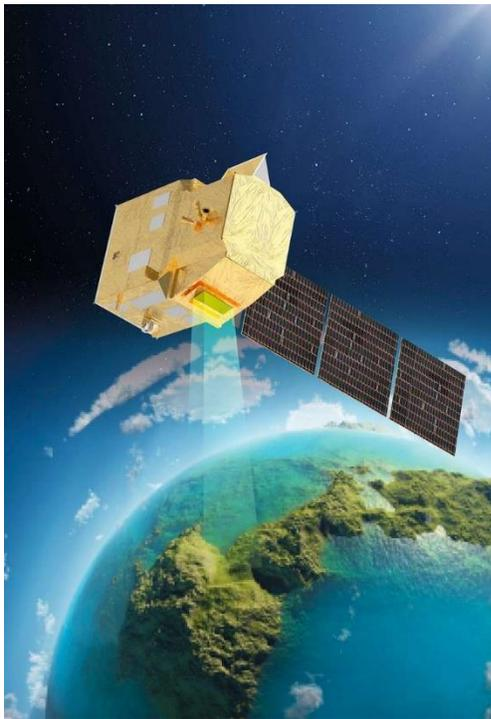
**Figure 1:** Copernicus Hyperspectral Imaging Mission for the Environment (CHIME), futur satellite Sentinel du programme Copernicus. © Thales Alenia Space
