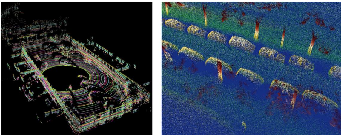
**Figure 6** : Point clouds acquired by the VELODYNE HDL-64E lidar (subsamped by a factor 50). **Left**: Points acquired for a single rotation. The points corresponding to the same laser head on the 64 laser rake are coloured in the same color. **Right**: Points corresponding to one section with multiple rotations. The colors of the points are height-coded. One can see that the occluded areas are rather limited.
