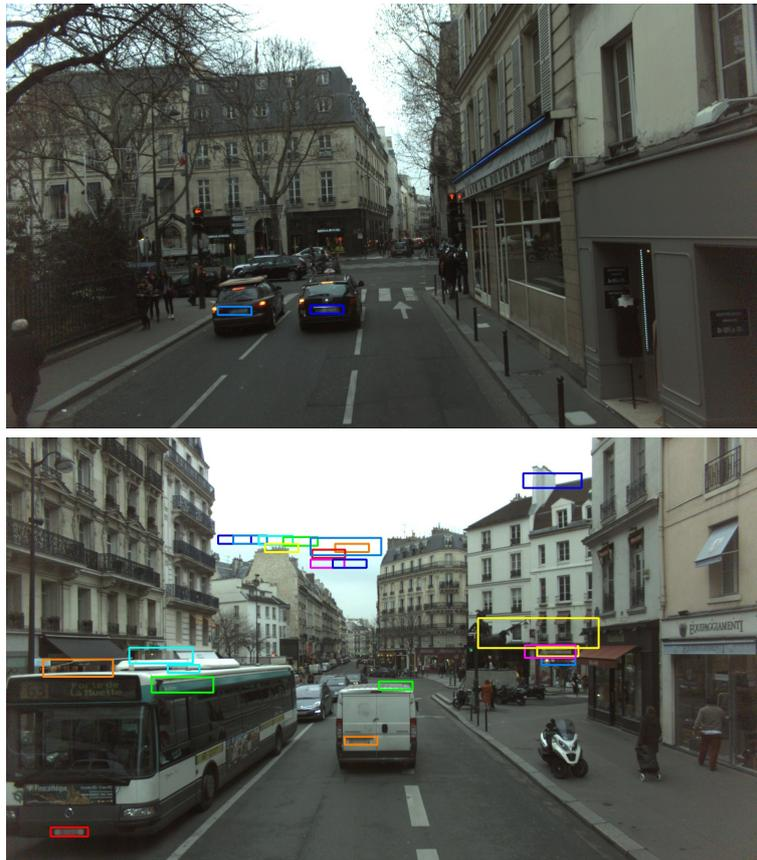
**Figure 17** : Results of car plate detection. One can see some false alarms, not yet filtered on a size criteria.
