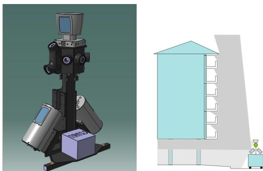
**Figure 5 :** **Left:**The rigid mount with the panoramic head, the IMU, the VELODYNE and the two RIEGL lidar devices. **Right:** Our acquisition geometry and coverage of the object space with the lidar sensors. The space covered by the RIEGL sensors and the VELODYNE are displayed in dark and light greys, respectively.
