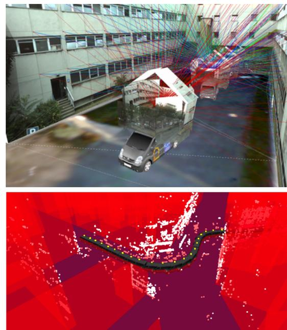
**Figure 11 :** Calibration of optical sensors with respect to the vehicle reference system. **Above:** Use of a network of surveyed targets fixed on building facades. **Below:** Self-calibration using natural details of the scene along the survey. A 3D model of the scene, displayed in red, is superimposed to the 3D measurements, in white, corresponding to the matched interest points. It qualitatively shows the satisfactory overall calibration procedure.
