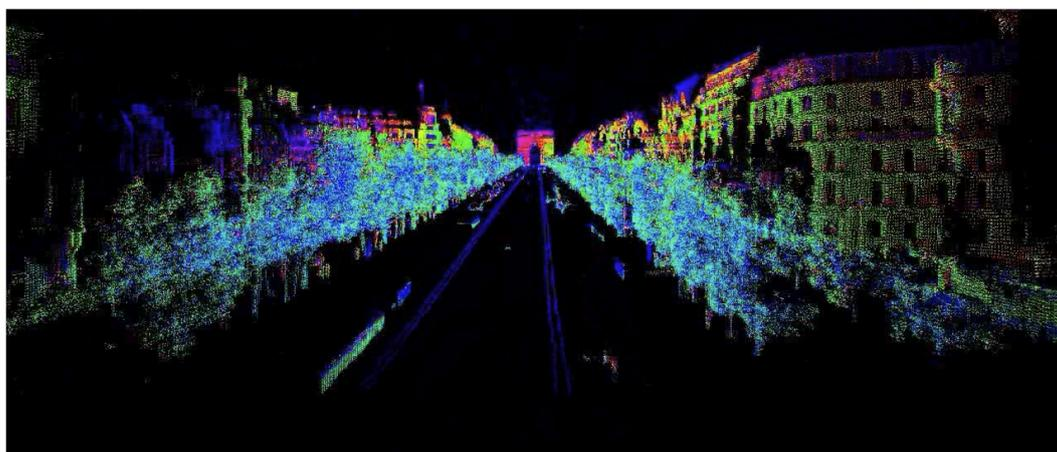
**Figure 8** : Point clouds acquired by the two upper RIEGL lidar devices (height colored) over the Champs-Élysées avenue, Paris, France.
