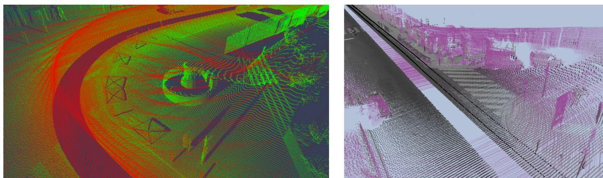
**Figure 7** : Point clouds acquired by the two RIEGL devices. **Left**: Acquisition of the bottom of a urban canyon. The 3D points are displayed in green. The rays corresponding to the path of the laser beam from the aperture to the measured surface are shown in red. One can see the important shadows due to the acquisition geometry. **Right**: Superimposition of laser point clouds of the VELODYNE (black) together with points of the RIEGL (pink).
