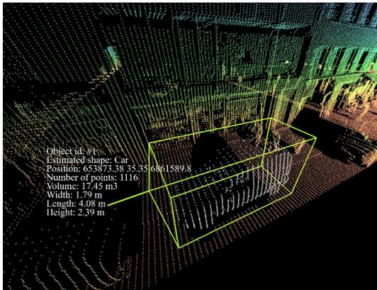
**Figure 14 :** 3D Bounding Box design and subsequent 3D point extraction (white), and statistics.
