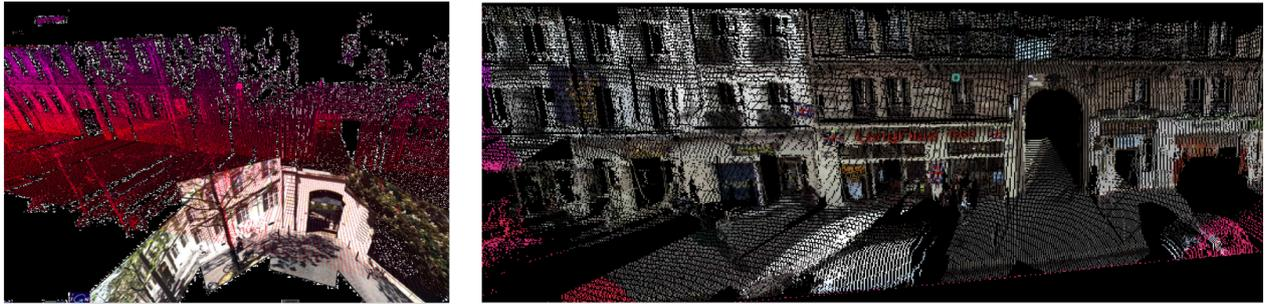
**Figure 12** : Relative calibration results of images with respect to the RIEGL lidar point cloud. **Left**: A panorama superimposed with the point cloud. **Right**: A 3D lidar point cloud colored with one of the referenced images.
