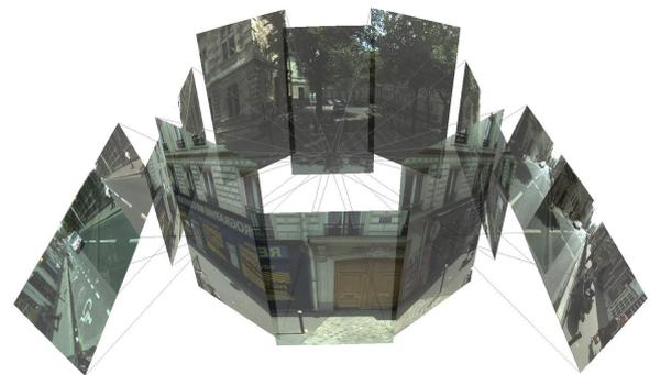
**Figure 4 :** The set of images acquired at one pose of STEREOPOLIS. One can see the images acquired by the panoramic head in the middle and also the images acquired by the stereo rigs on the left and on the right of the Figure. Each image is full HD.
