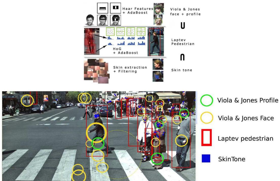
**Figure 15 :** Pedestrian extraction. **Left:** The pedestrian detection system. **Right:** Results of the four detections on a sample of one image.
