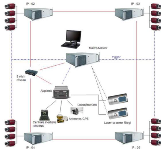
**Figure 9 :** **Left:** Back view of the STEREOPOLIS system. One can see the five personal computers (PC) used for processing and storing the acquired imagery. **Left:** The global system architecture of STEREOPOLIS.
