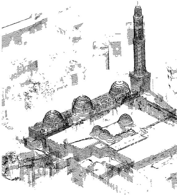
**Figure 8 :** Automatically computed cross-sections in laser 3D points of the mosque Al Muzzafar in Taz (Yemen).
