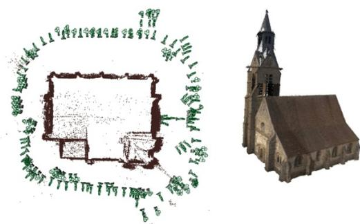
**Figure 10 :** 3D model on the Rampillon church near Paris produced by Micmac (the left image shows the camera positions).
