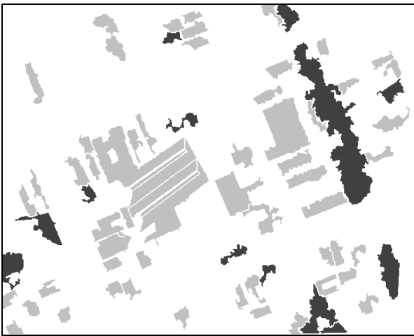
Figure 4: Trees (dark areas) separated from buildings (light grey) using the vegetation index.
