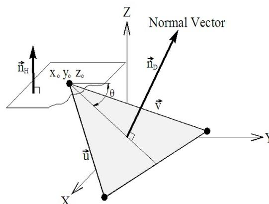
**Figure 2:** Delaunay triangle of a hypothetical horizontal plane.
