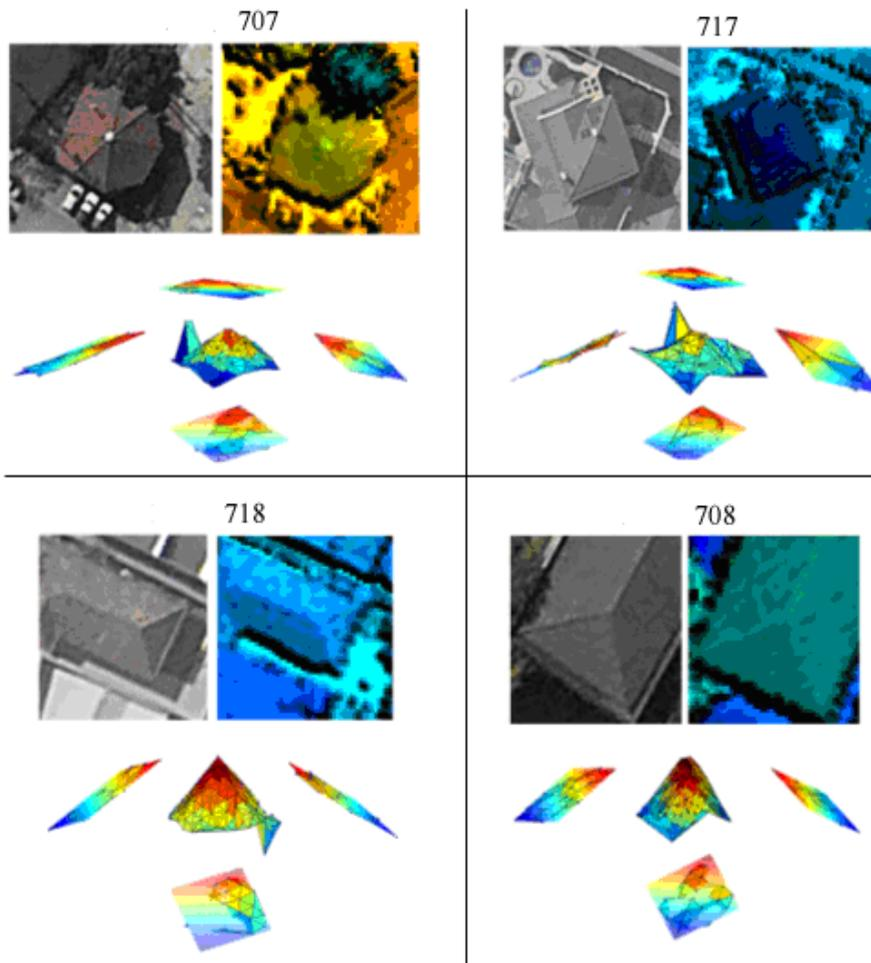
**Figure 8:** Sloped roofs extracted semi-automatically in aerial photograph, laser scanning intensity image and laser scanning hard data and adjusted planes.
