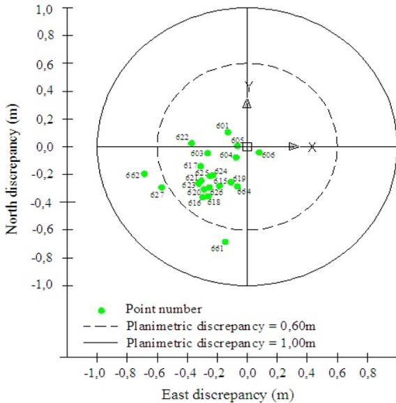
**Figure 9:** Planimetric discrepancy of GPS coordinate of pre-signalized points and the ones obtained from phototriangulation supported by laser scanning points.
