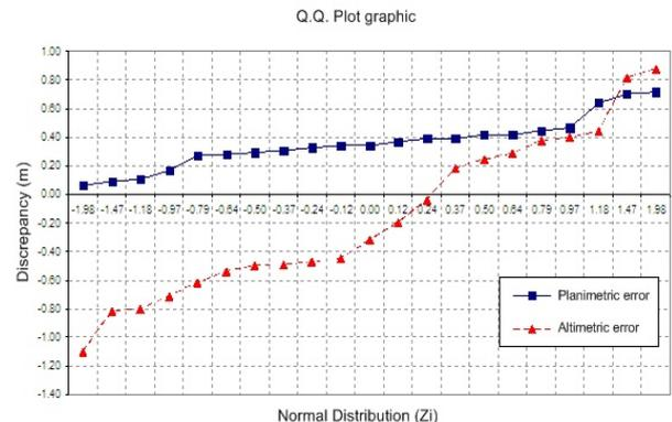
**Figure 11:** Q.Q. Plot graphic for the Filliben test in its planimetric and altimetric component.
