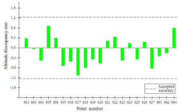
**Figure 10:** Altimetric discrepancy of the pre-signalized GPS points and the ones obtained from phototriangulation supported by laser scanning points.
