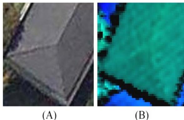
**Figure 1:** Building roof present in (A) aerial photography, and (B) in the laser scanner intensity image.
