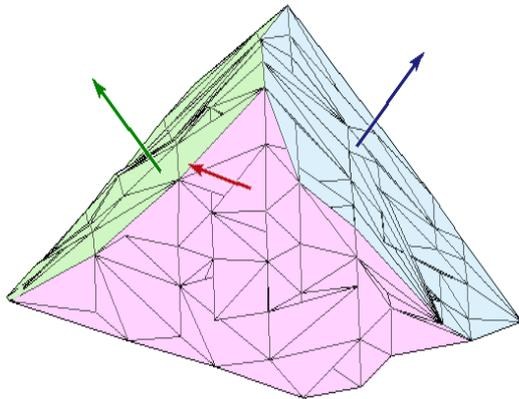
**Figure 3:** Delaunay triangulation which represents different sloped roofs.
